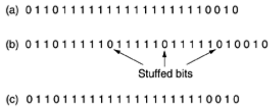
Fig: Bit stuffing. (a) The original data. (b) The data as they appear on the line. (c) The data as they are stored in the receiver's memory after destuffing.
